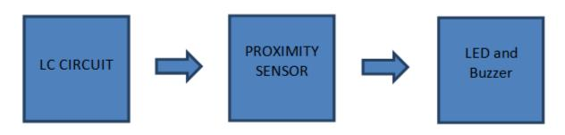
The LC circuit is nothing but inductor and capacitor which is connecter in parallel. The LC circuit will trigger the proximity sensor if it detects any metal near to it. Proximity sensor will give glow the led, and also make the buzz with the help of the buzzer.
